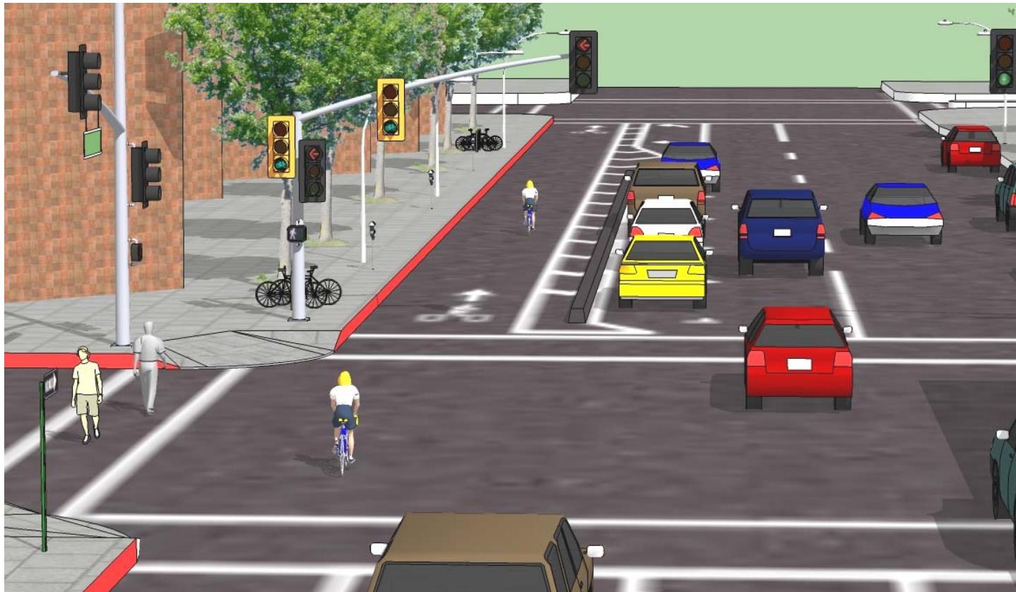
Typical design configuration for the protected bikeway; Bikes and vehicles going through Third Street & Broadway have green lights
