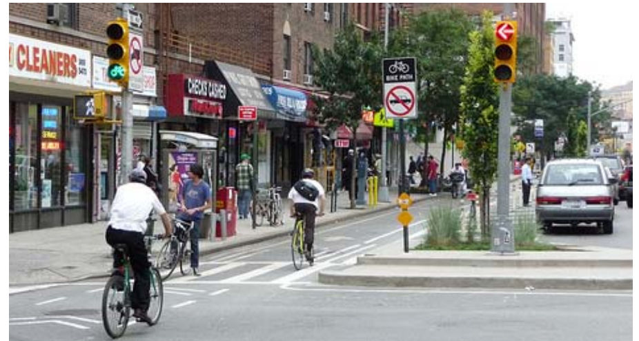
Protected bike lane located on the left side of the roadway in New York City
