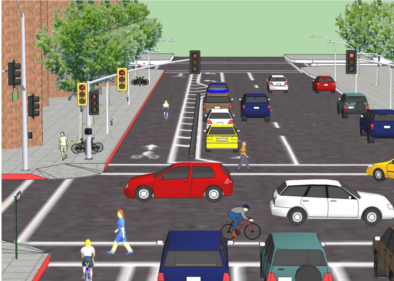
Typical design for the protected bikeway. Bikes and vehicles going through Third & Broadway stop for cross street traffic
