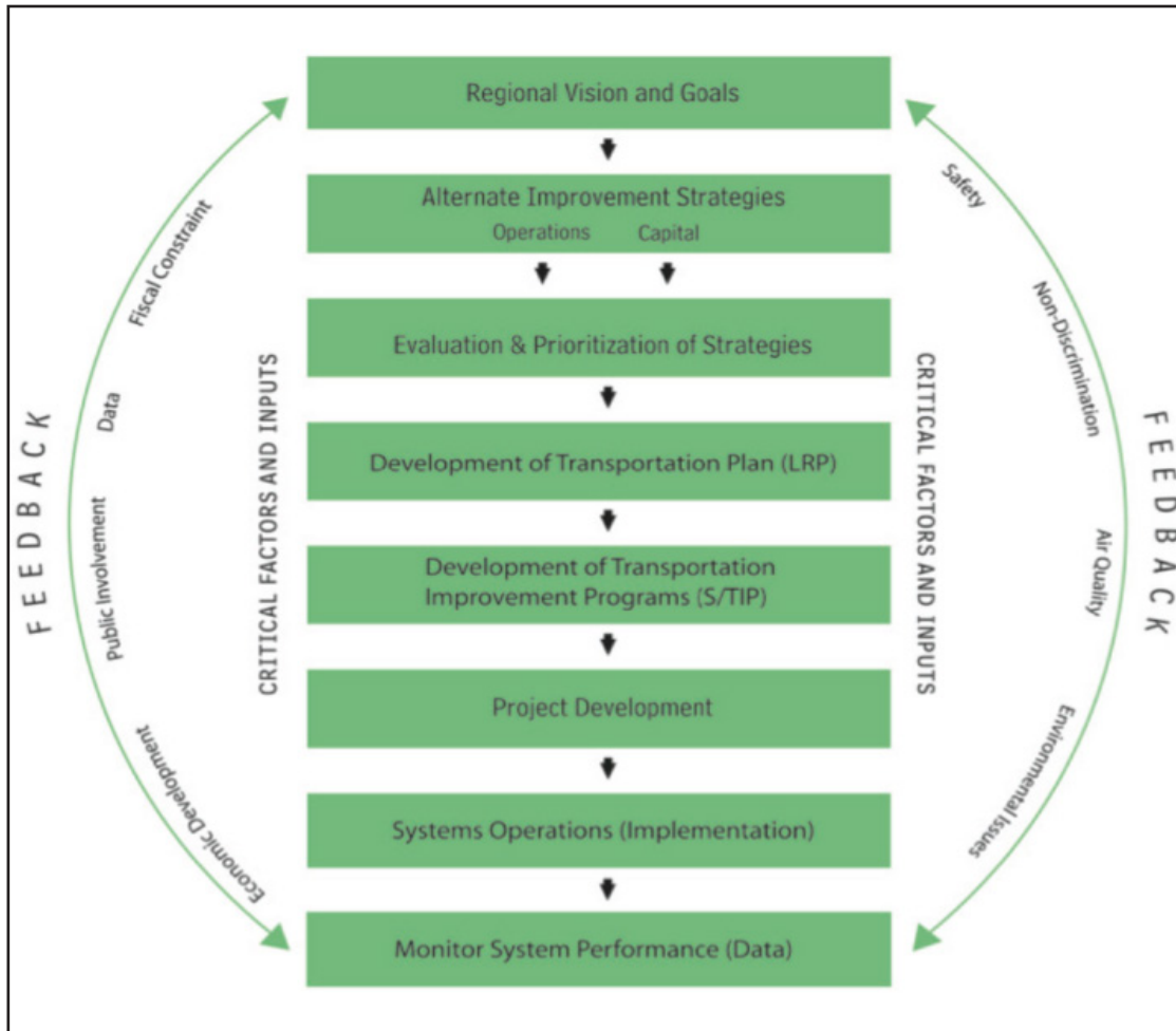
FIGURE 7. DEVELOPMENT OF A PROJECT 29
