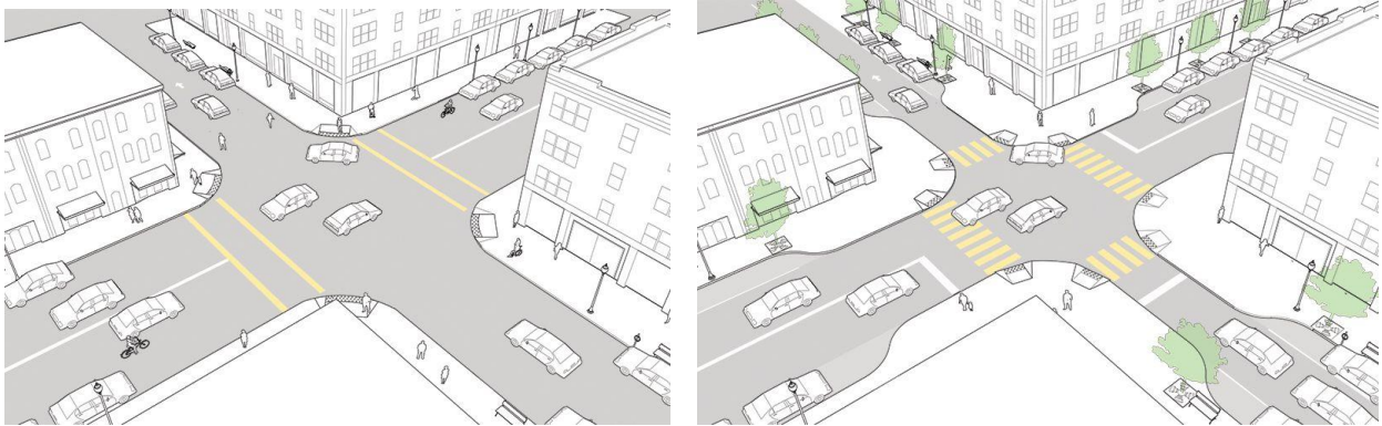
On left, “standard” crosswalk striping; on right, high-visibility “continental” crosswalk striping Renderings courtesy of NACTO.org
