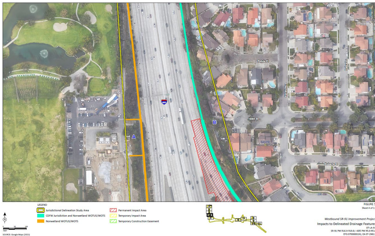
Figure 1: Impacts to the upper portion of Drainage Feature B.
