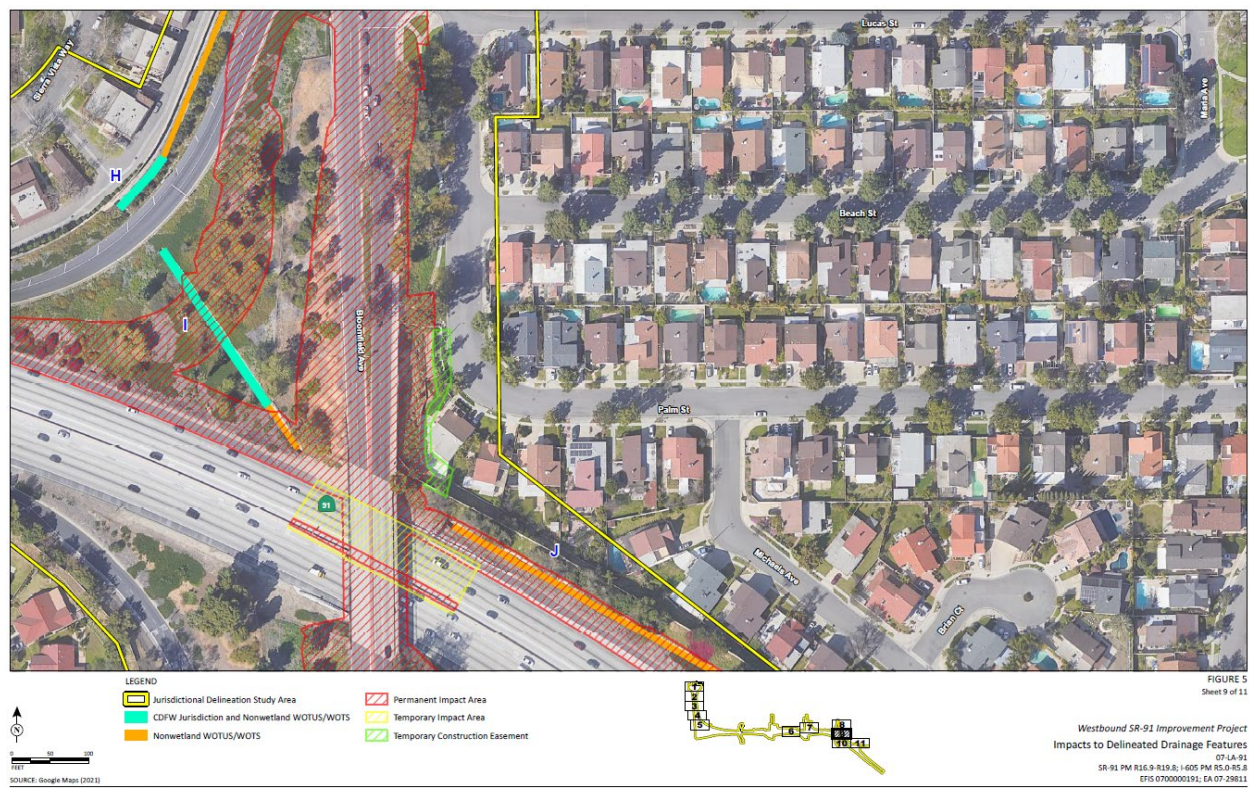
Figure 4: Impacts to the upper portion of Drainage Feature I and Drainage Feature J.
